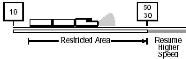
[Diagram G. Displaying Permanent Speed Restriction Signs.]
